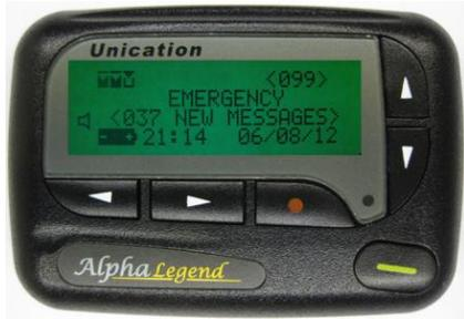
To access – push Function button ● from the Home screen. ( this key has a different function set in the message screen)
